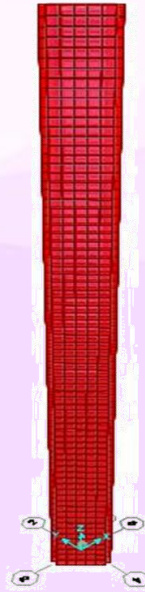
Figure 2: Square Stone Chimney Finite Element Model without CFRP
