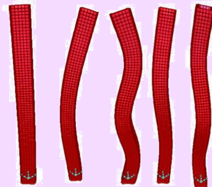
Figure 3: Respectively Mode Shapes of Square Stone Chimney without CFRP
